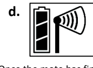
Once the mote has finished joining the network, the "x" icon is removed and the channel count on the station LCD increases by three (two for water potential and temperature, and one for the mote battery).
