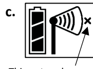
This network connection "x" icon blinks while the mote completes the registration process, which may take up to five minutes.
