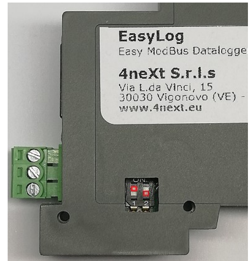
Fig. 6 DIP Switch position for DHCP
